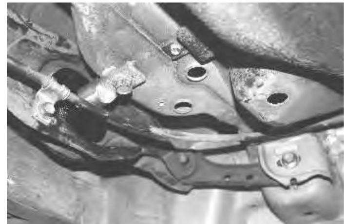
10. Insert supplied aluminium pin and bolt to chassis, no grease is required - see image 7.
