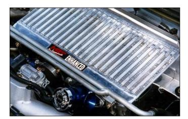
Before a big dose of boost was injected to wake the engine up, an MRT replacement top-mount bar-and-plate air-to-air intercooler (and associated water spray) was slipped in before the throttle. Bolted to the engine side end-tank is a GFB (Go Fast Bits) atmospherically venting blow-off valve.
