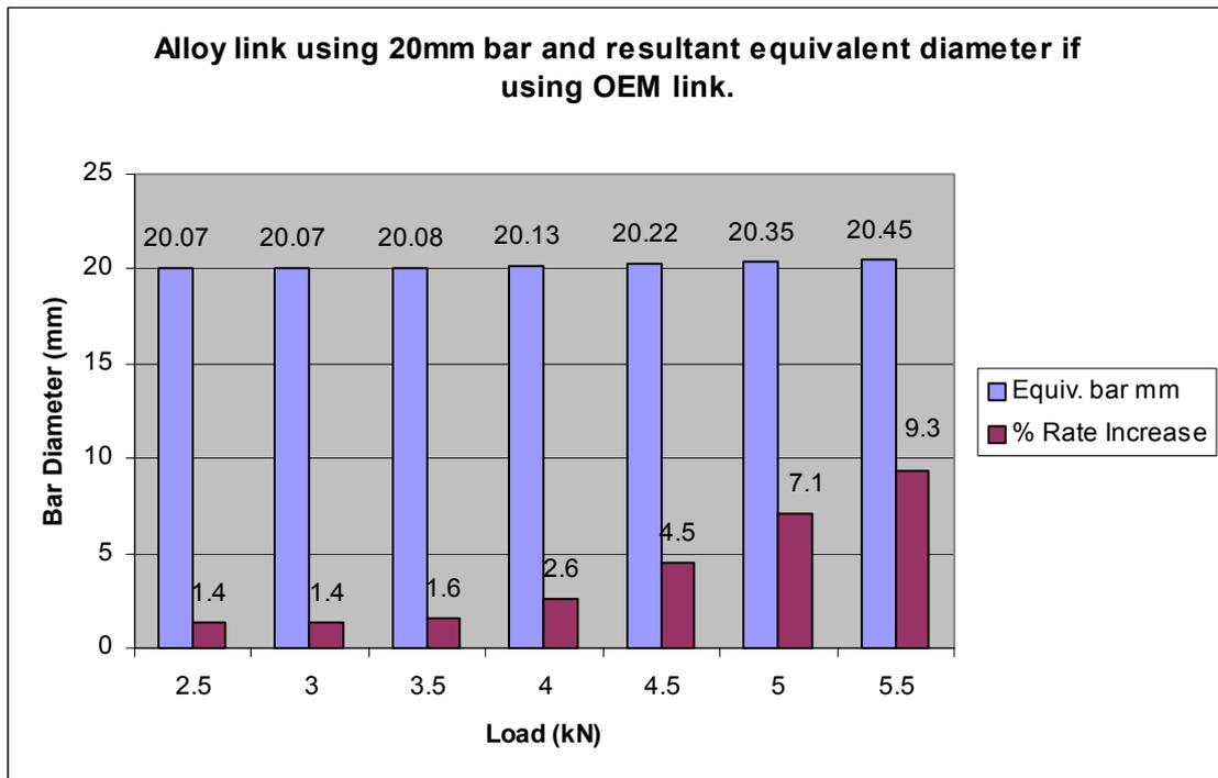
This table clearly shows a relatively insignificant change in anti-roll effect when using standard or relatively small bar diameters even at high cornering loads.
