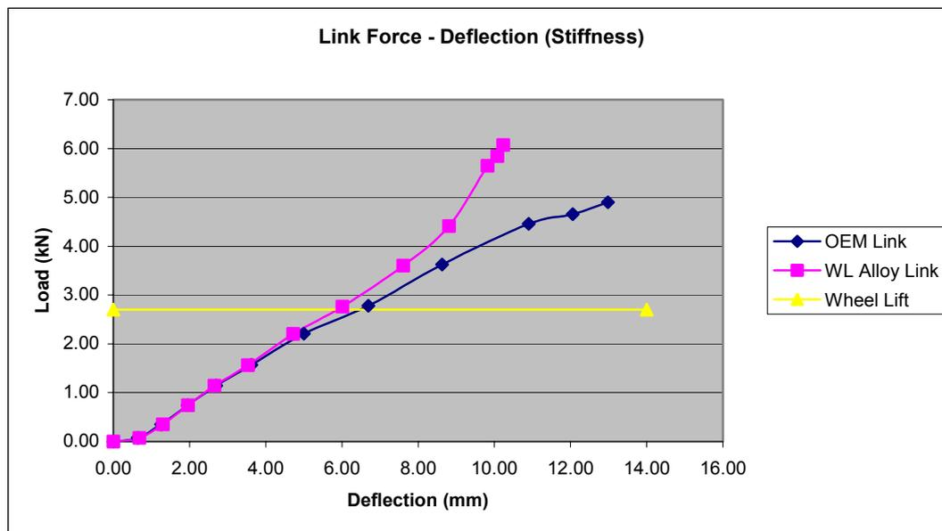
This value (2.7 kN) was calculated from “Race Car Vehicle Dynamics” (Milliken & Milliken) roll rates for “firm high (performance imports)” using the standard suspension geometry. For more heavily modified “track cars” running larger diameter bars (24mm) and cornering up to 1.2g, the load transmitted through the link would be approx. 3.5 kN. If momentary peak cornering loads were also to be assumed, say around 1.5g cornering, this would incur loads of up to 4.5 kN (for track cars).
