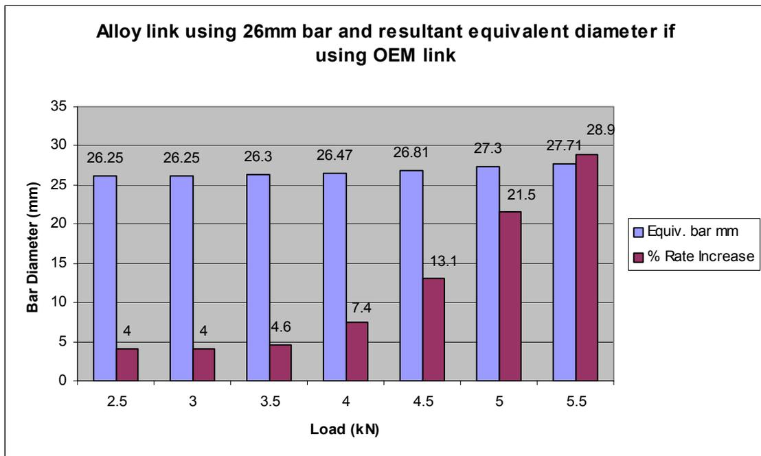
As can be seen in the three graphs, as the load increases the effect of the extra stiffness in the alloy link increases. This is because of the alloy link stiffness profile being stiffest at higher loads.
